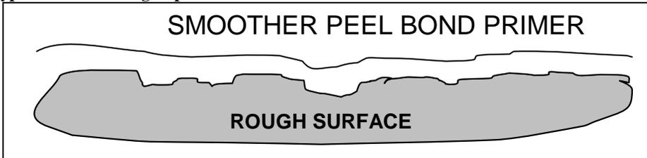
**NOTE:** Remove all loose and peeling paint. The surface should be a sound, stable surface. Spot prime areas that require extra filling. The moisture content of wood should be **Below 15%** at application.
